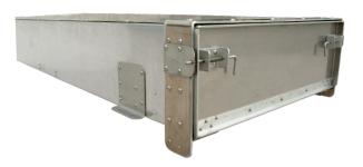
We also make under truck carriers for the ramps made from extruded aluminum. These carriers have stainless steel brackets so you can bolt or weld them under the trailer. These carriers will be about 100 lbs. lighter than steel carriers and will not rust. If you have any questions please call us at 419-923-7353.
